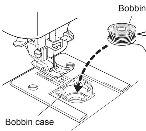
Thread unwinding direction
