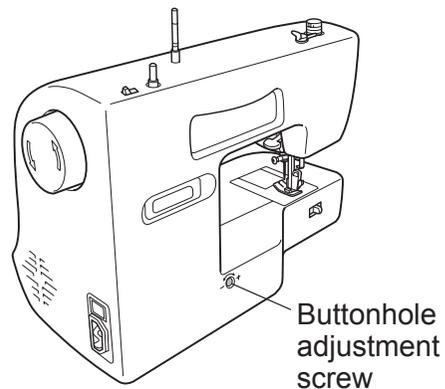
If the stitches are loose on the right side of the buttonhole, turn slightly in the “-” direction.
