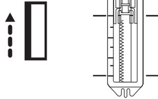
**5** Raise the needle to the highest position, set the pattern dial to “2”, and sew 5 to 6 bar-tack stitches. “2” and “4” on the pattern selection dial use the same dial position.
