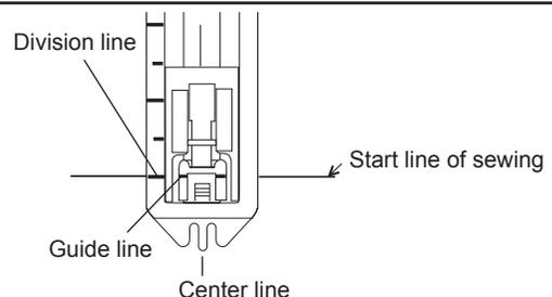
**4** Raise the needle to the highest position, set the pattern dial to “1”, sew the left side and stop at the line marked on the fabric.
