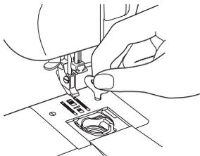
**3** Lift up the bobbin case so that part ③ is moved past part ④, as shown.
