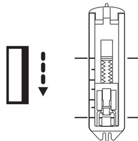
**7** Raise the needle to the highest position, set the pattern dial to “4”, and sew 5 to 6 bar-tack stitches.
