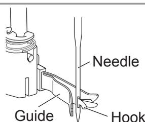
The hook is within the guide. The hook passes through the needle, catches the thread, then pulls the thread through the needle.
